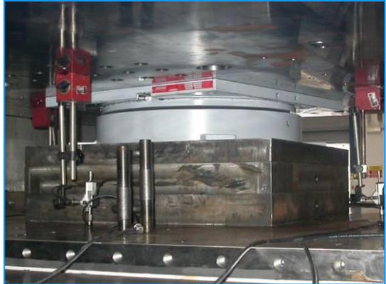
**Agom V-max bearing during friction test**
